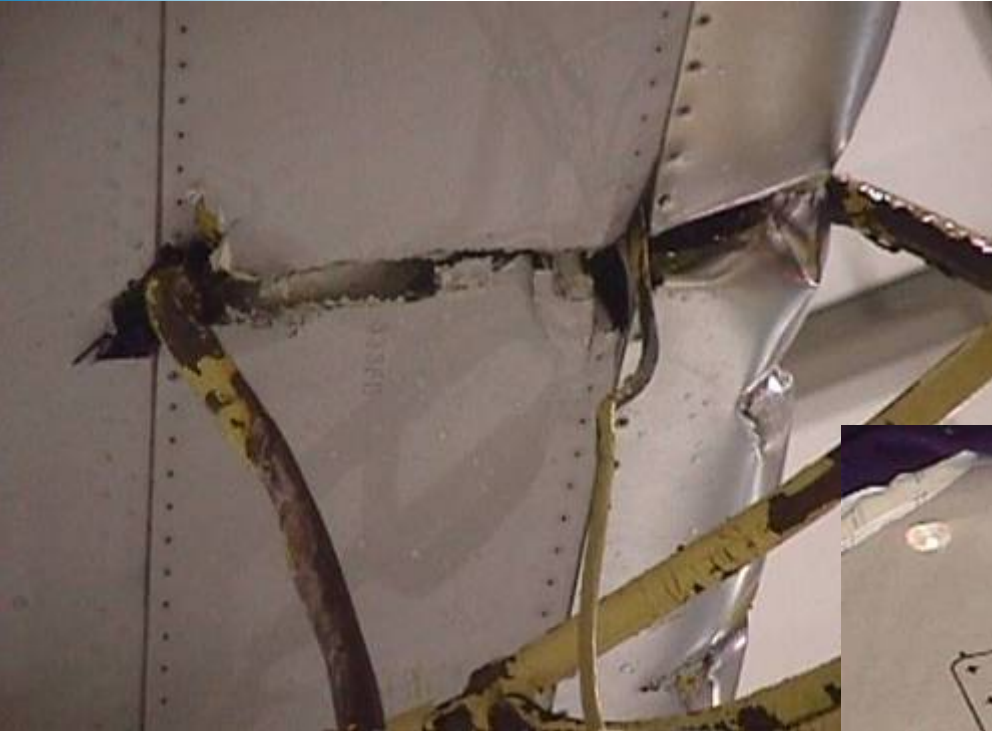
Skin/Spar Damage—Ground Handling Equipment Impact
